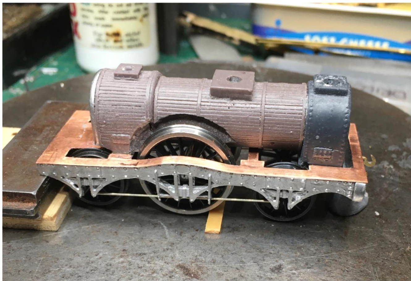
The copper sheet footplate and 'too big' cut out of the boiler to accommodate OO wheels, the gauge of which is too narrow (but let's not start that discussion...!).
