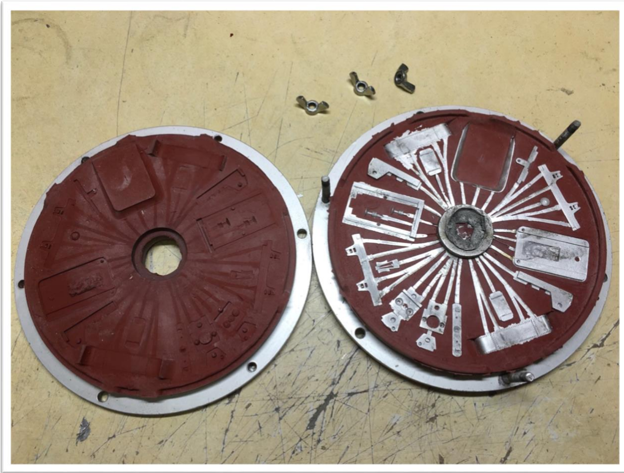
The cast tender 'kit' ready to be released, cleaned up, and assembled.
